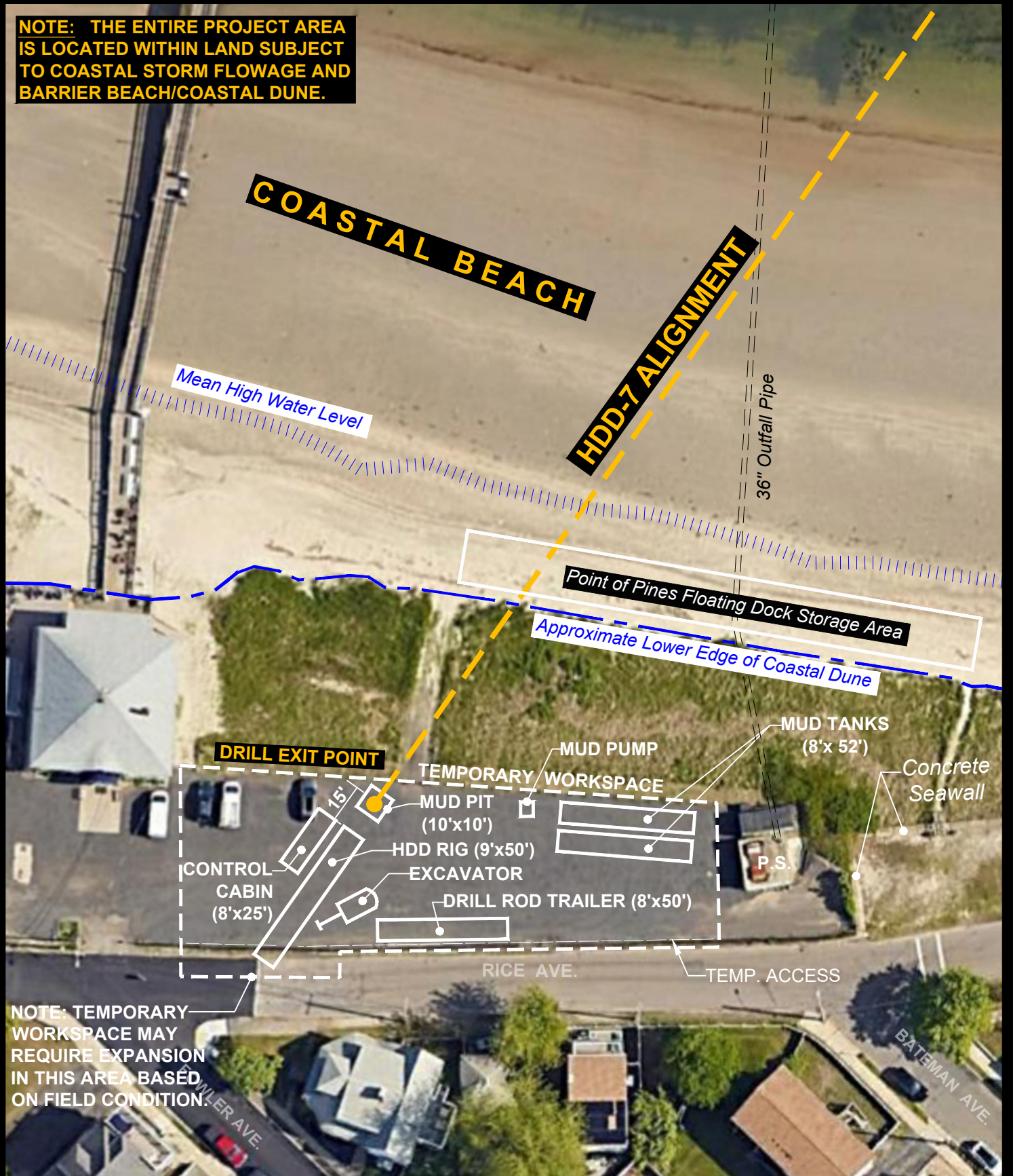
FIGURE 6.1-5B HDD-7 EXIT POINT (MAJOR EQUIPMENT - PIPE PULLBACK PHASE) SAUGUS RIVER CROSSING - REVERE, MA June 2023
