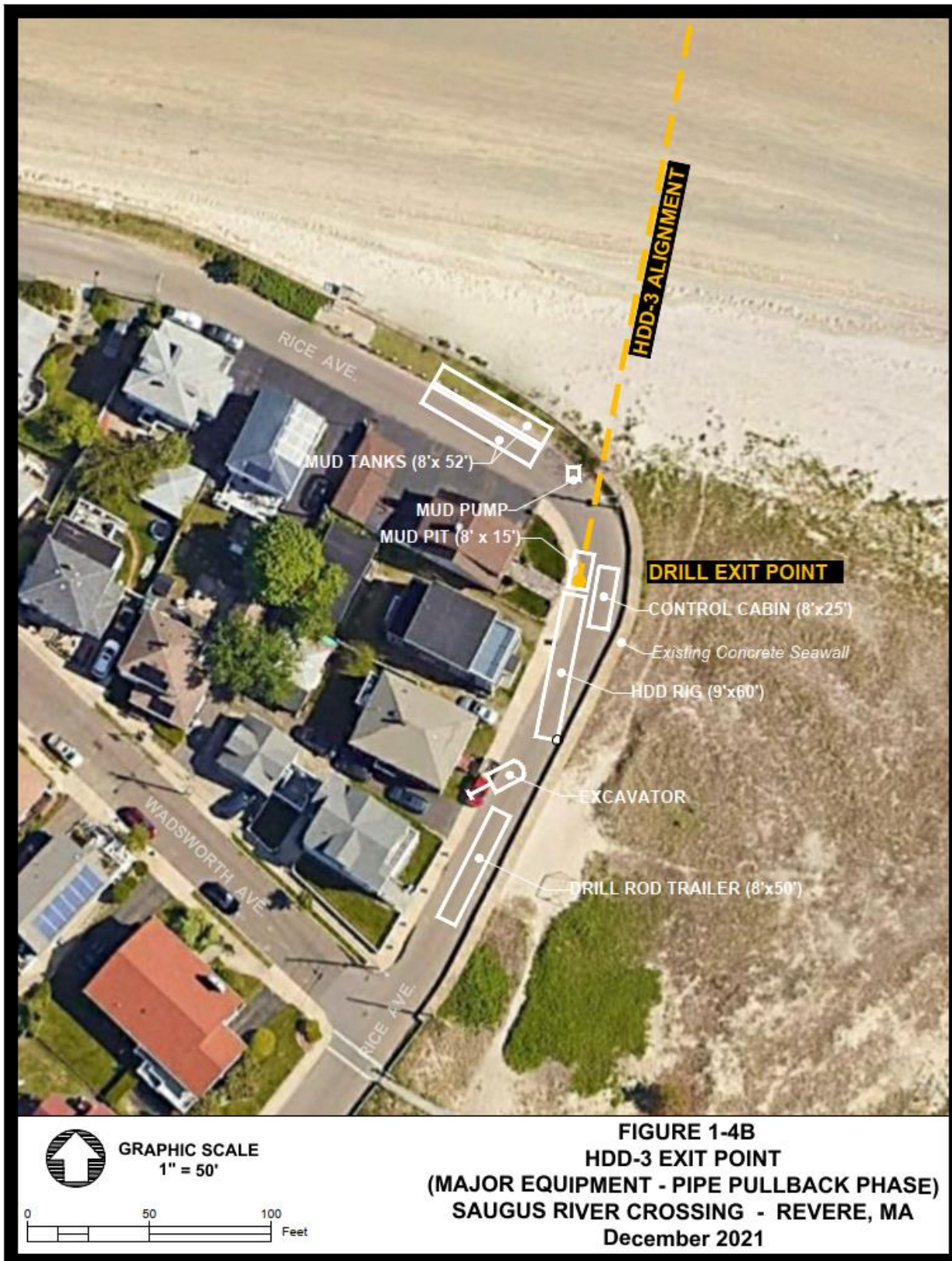
Figure 3 - Equipment Staging for HDD Route 3
