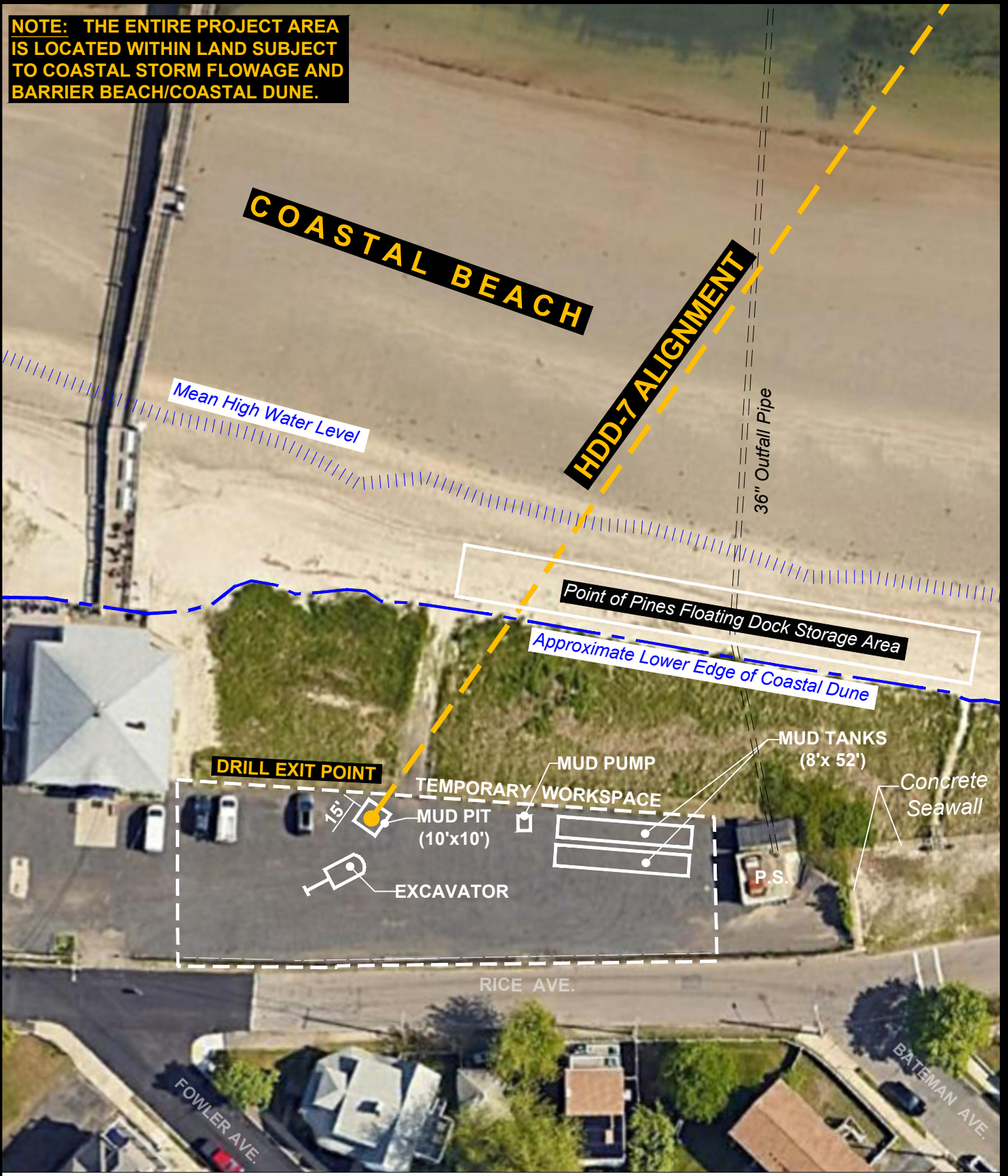
FIGURE 6.1-5A HDD-7 EXIT POINT (MAJOR EQUIPMENT - DRILLING PHASE) SAUGUS RIVER CROSSING - REVERE, MA June 2023
