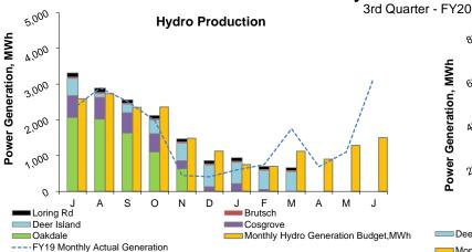
In the 3rd Quarter of FY20, the renewable energy produced from all hydro turbines totaled 2,301 MWh; 11% below budget³. There were no Quabbin Tunnel transfers during the quarter. The total energy produced to-date in FY20 is 15,518 MWh; 2% above budget³.
