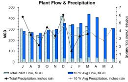
Total Plant Flow for the 3rd Quarter was 14.0% below target with the budgeted 10 year average plant flow (326.7 MGD actual vs. 379.8 MGD expected) as precipitation was 24.6% below target (8.29 inches actual vs. 11.0 inches expected). Total Plant Flow was 10.1% lower than the 4 year average plant flow used for energy budget projections.
