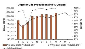
The Avg Daily DiGas Production in the 3rd Quarter was 3.6% above target with the 2 Year Avg Daily DiGas Production. On average, 99.4% of all the DiGas produced in the quarter was utilized at the Thermal Power Plant (TPP).
