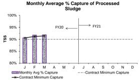
The contract requires NEFCO to capture at least 90.0% of the solids delivered to the Biosolids Processing Facility. The average capture for the 3rd Quarter and for the first three (3) months of CY20 was 91.4%.
