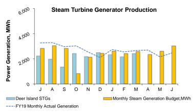
In the 3rd Quarter of FY20, the renewable energy produced from all steam turbine generators totaled 6,871 MWh; 9% below budget<sup>3</sup>. The total energy produced to-date in FY20 s 19,472 MWh; 10% below budget<sup>3</sup>. The total savings and revenue<sup>2</sup> to date in FY20 (actuals through February<sup>1</sup>) is \$1,672,605; 15% below budget<sup>3</sup>. The savings and revenue value does not include RPS REC revenue (see next page).
