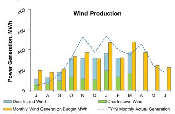
In the 3rd Quarter of FY20, the renewable energy produced from all wind turbines totaled 1,059 MWh; 17% below budget<sup>3</sup>. The total energy produced to-date in FY20 is 2,417 MWh; 16% below budget<sup>3</sup>.
