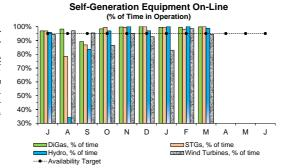
The DiGas system, STGs, and Hydro Turbines all met or exceeded the 95% availability target for the 3rd Quarter. Wind Turbine availability was just under target by 3.1% due to brief periods of downtime from a combination of mechanical issues and turbulence caused by wind blowing through the digesters, tripping the turbine out of service.
