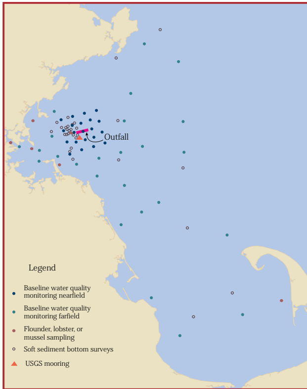
Figure 24. Monitoring stations include water, sediment, and the biota close to and distant from the new outfall site.
