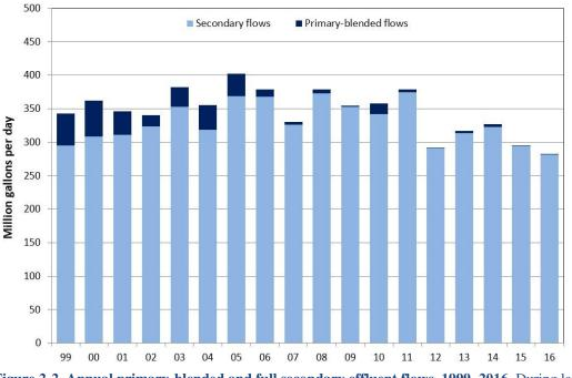
**Figure 2-2. Annual primary-blended and full secondary effluent flows, 1999–2016.** During large storms, flow exceeding the secondary capacity of the plant is diverted around the secondary process. Primary-treated flows are blended into secondary-treated flows before discharge.
