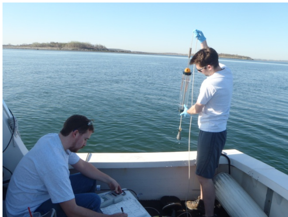
Fig. 4. Water sample collection using a Niskin bottle.
