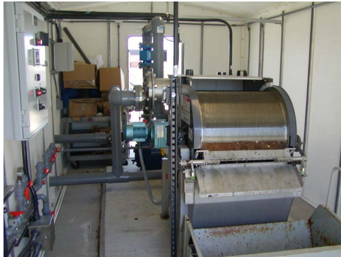
Figure 1. Effluent floatables sampling device
