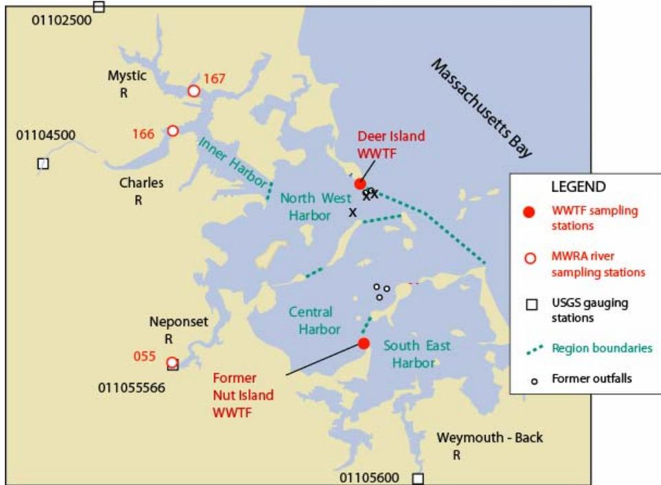
Figure 2. Stations at which flows/loadings were measured. 'x' marks the locations at which sludge was discharged prior to 1991.
