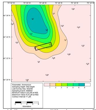
Figure 6-2. Horizontal contour of  $NH_4$  at the pycnocline. The rectangle represents the location of the diffuser.
